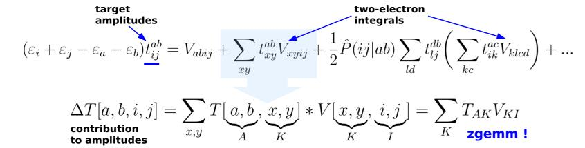
FS-RCC = matrix-matrix multiplications + "tensor" transpositions
